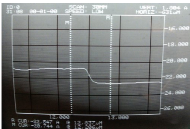
Step of 180 nm Aluminum on float glass – Zoom on Step
