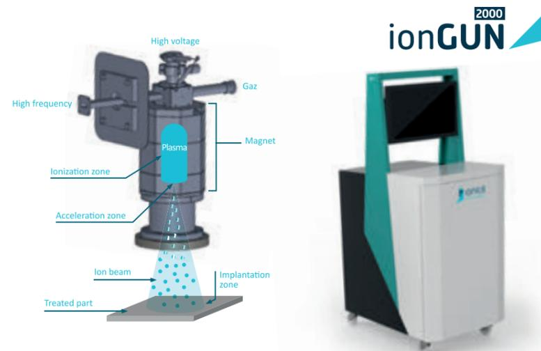
A micro-accelerator of particles generates a highly energetic ion beam able to penetrate the surface of materials and to enhance their properties without any coating.
